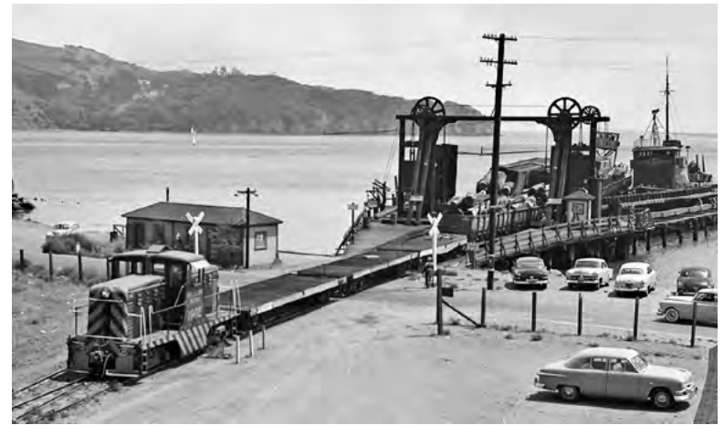
NWP's first diesel engine #1902 loading lumber cars onto a barge in 1953. The three flat cars are to keep excess weight off the gallows apron. (Codoni collection)
