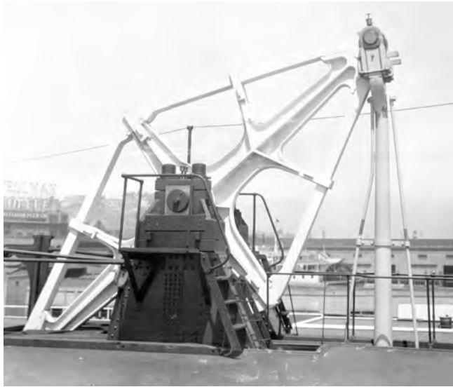
A typical walking beam structure that powered the paddlewheel ferries.
